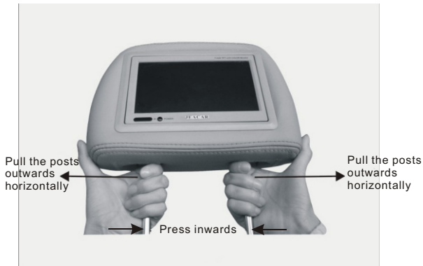
3. Pull the posts outwards horizontally
